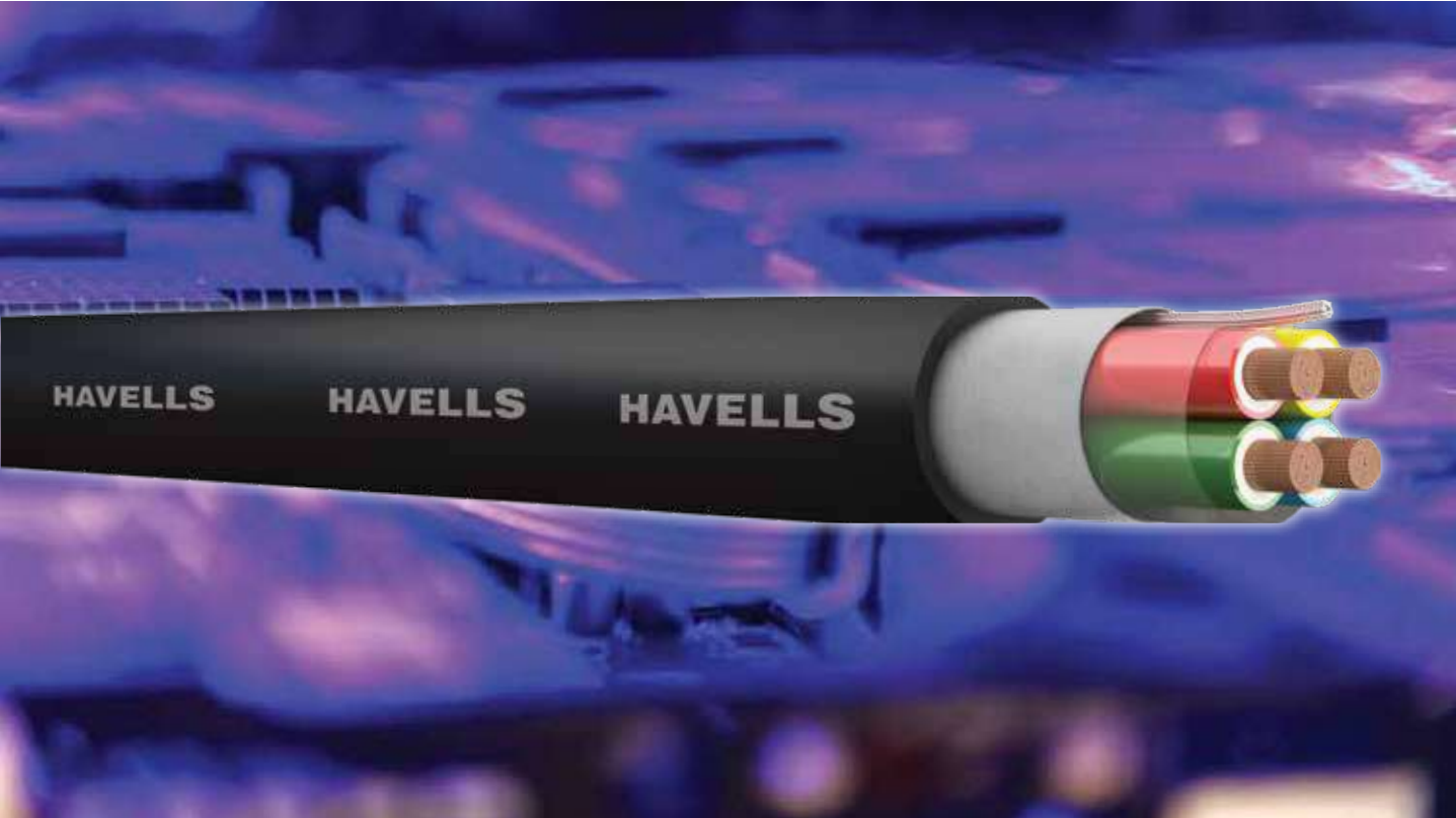
Havells 1100 Volt Flexible ABC Conductor, PVC Type D Insulated, Cores laid up, Overall Shielded by Al-mylar along with ATC drain wire & Overall PVC Type ST-3 Sheathed Cable HSN CODE: 8544
