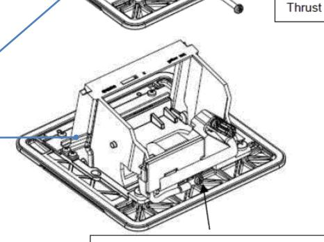
To fix the support by making earthing
